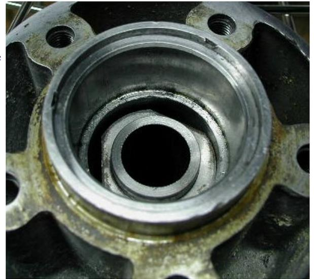
You can press this bearing into the hub the same way as the other bearing, making sure you keep the spacer aligned or you can build a drift by taking two 7/16" washers just under the size of the O.D. of the bearing, relieving the center of one washer, and using the front wheel spindle. This picture shows the two washers with one relieved so as not to touch the inner race of the bearing.
