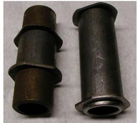
Both spacers have pressed fitting flanges that are easily removed by placing the inside part of the flange between two flat surfaces (like the jaws of a vise) and gently pounding the spacer down. The picture shows the spacers with the flanges removed.
