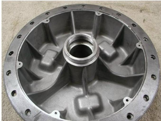
This hub has a stepped spacer that allows the bearings to be driven out by inserting a drift in one end and pressing the spacer through the hub. Since the end of the spacer, where the threaded cap is inserted, sticks out beyond the bearing, it is easier to drive the spacer from this end.
