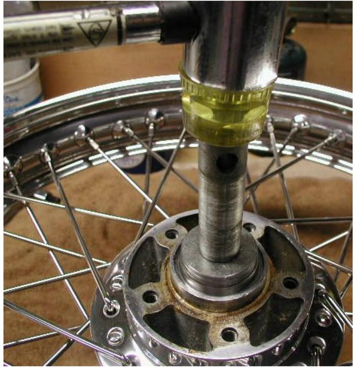
This picture shows bearing inserted into the hub.
