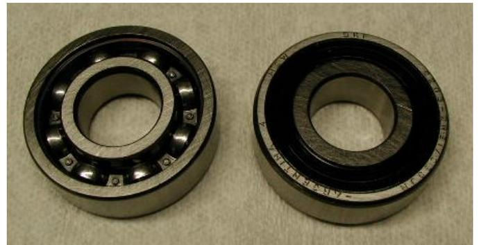
On the disc side a double row bearing is used and this picture shows the stock bearing (part # 06-7688, \$X.XX) which is a 17x40x16mm bearing or .6299" thick, on the left and the sealed bearing (part # 06-7688/S, \$X.XX) which is a 17x40x17.42mm bearing or .6858" thick, on the right. You will notice that the sealed bearing is slightly thicker than the stock bearing (.0559" thicker or .056").
