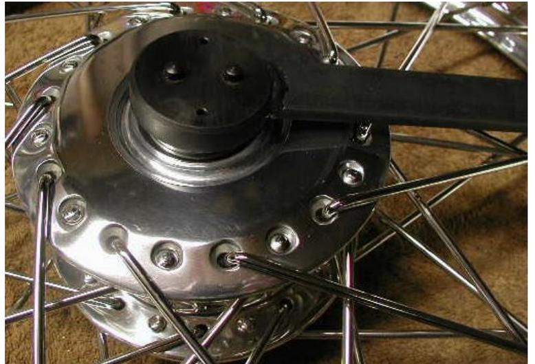
I found that if you leave the felt seal (06-7614) out, the wheel will spin freer and by using a sealed bearing the felt seal is redundant. After saying this I have found, on the earlier hubs, the felt seal does help with spacing so it is your call. This picture shows the non-disc side assembled without the felt seal.
