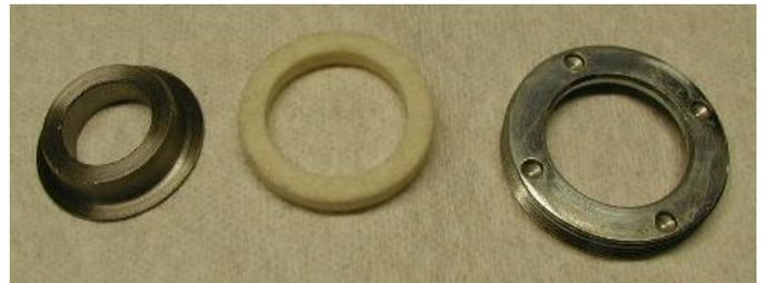
These parts are assembled in the order shown with the spacer fitting down on the wheel bearing, the seal fitting around the spacer and the lockring screwing into the hub.
