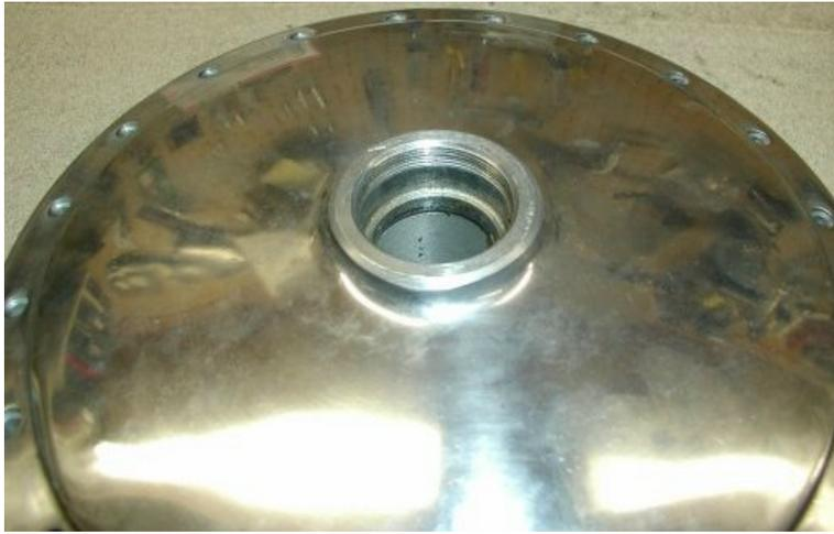
This picture shows the front drum hub, non brake side and the next picture shows the brake side. Removing the bearings from this hub is done just like the front disc hub described above. The double row bearing is on the brake side.
