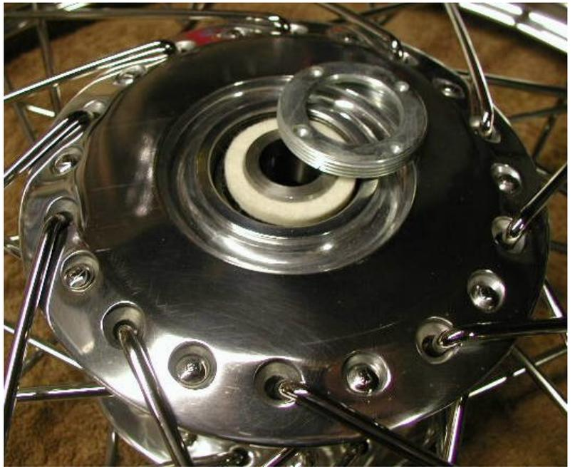
The Lockring is tightened by using the factory spanner ( [06-3965](#) ). The current price for this spanner is \$X.XX.
