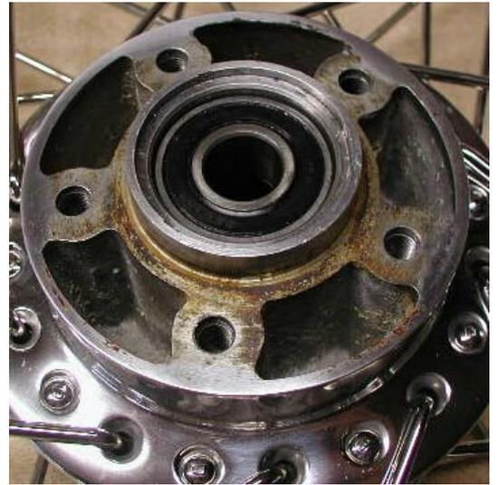
You can assemble the washer (06-2071), felt seal (06-7614) and retaining washer (06-7751) or leave them out depending on your preference.
