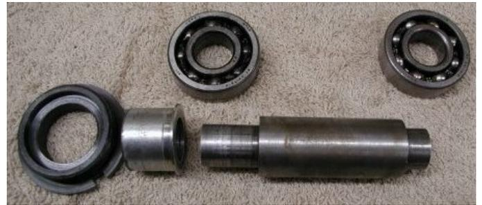
The drift shown here is our drift number CD-0002 (for drift dimensions see drift number [CD-0002](#) in our drift information page), but could be any rod that is slightly smaller than the bearing bore, but larger than the I.D. of the spacer end.
