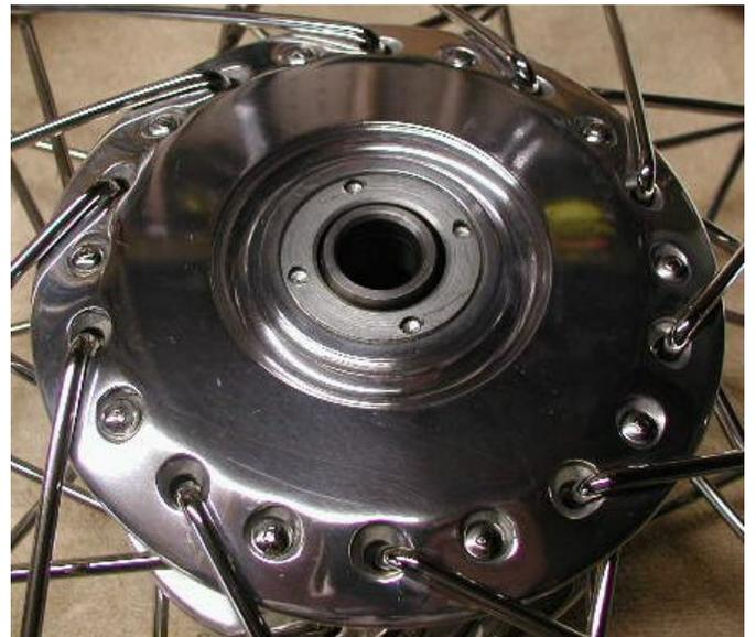
**Fitting the disc side bearing:** This is the side that requires some modification in order to upgrade the stock double row bearing with a sealed bearing. This picture shows the bearing spacer (part # 06-1955, \$5.80) with the new spacer on the left and an older spacer on
