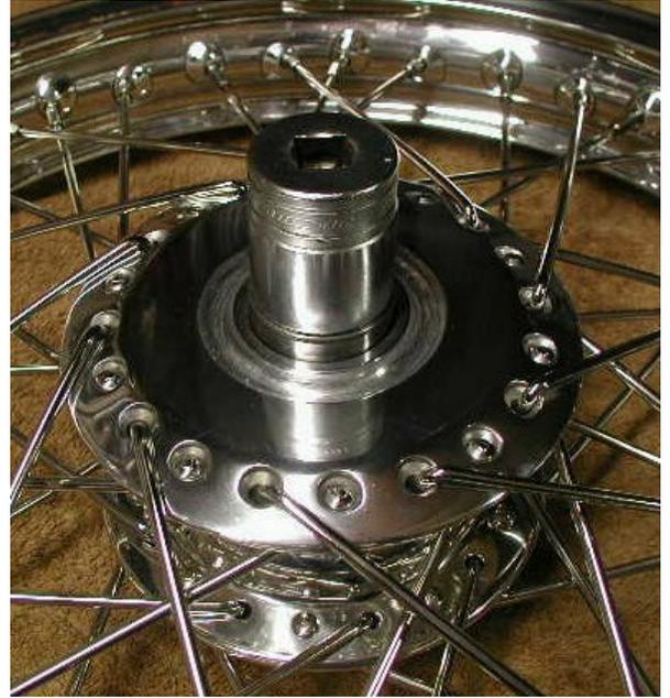
This next picture shows the bearing fully pressed into the hub.
