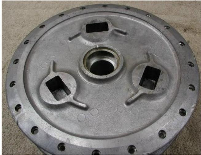
This picture shows the rear drum hub, drive side and the next picture shows the non-drive side.
