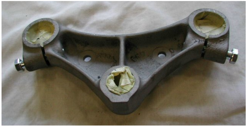
Two handlebar clips, part number 06-7727.
