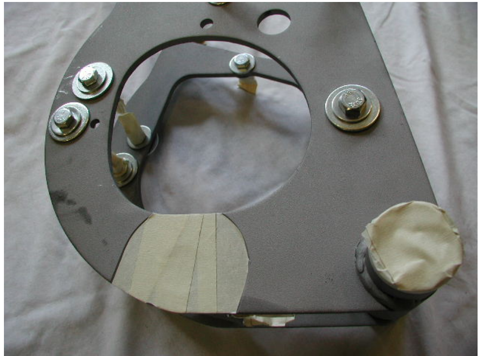
MK3 front engine mount, part number 06-5510.
