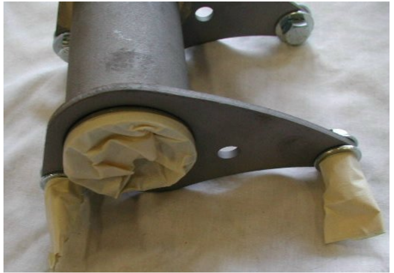
MK3 Rear caliper mount, part number 06-6206.
