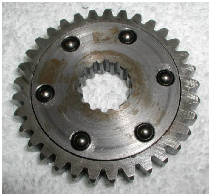
Place the carrier in the gear.
