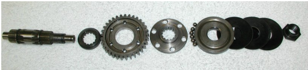
All the parts included in the backfire assembly.
