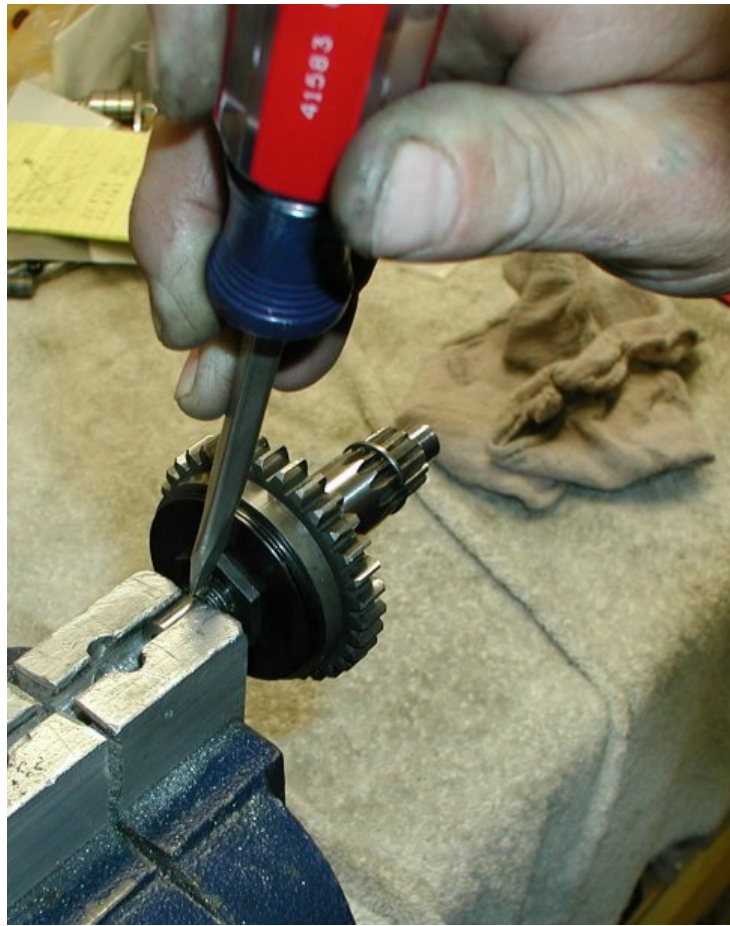
Peen in the nut flange.
