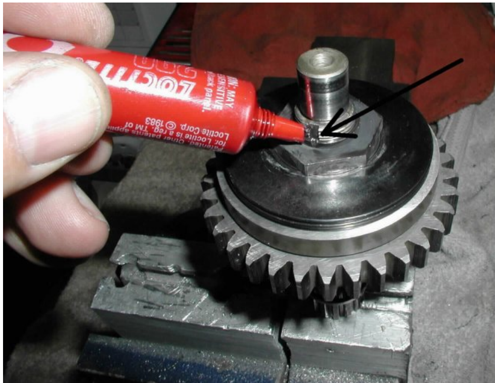
Use green loctite on the nut.
