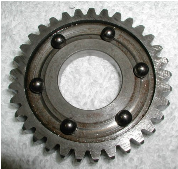
Place the six balls (06-4743)) in the gear.
