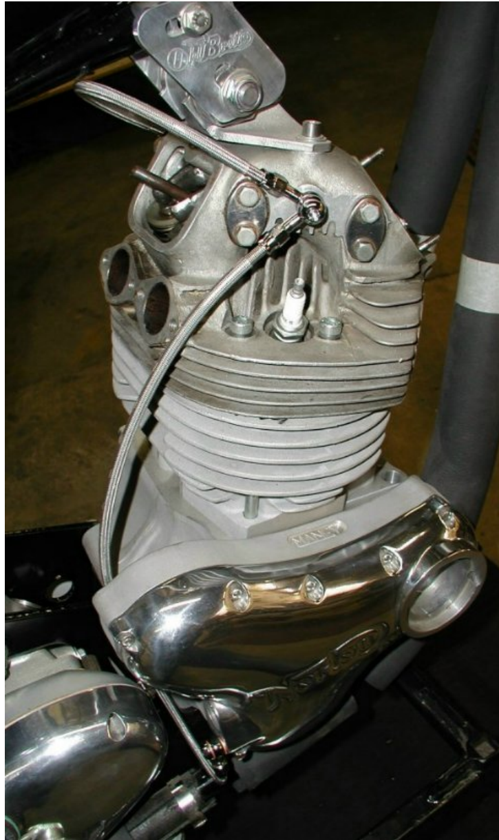
Rocker feed lines installed on an engine.
