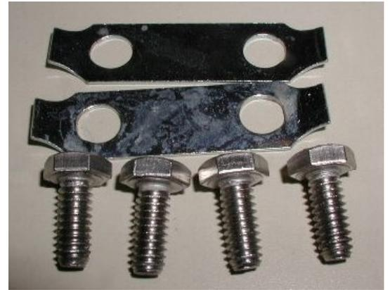
The tabs spread the bolt pressure across the fender flange instead of just around the bolt holes and they prevent the bolts from coming loose. These are factory tab washers used to secure the Oil Filter Housing, but work great for securing the fender. The holes on the tabs do need to be elongated slightly to match the slightly longer hole spacing on the slider. The tabs in this picture have been modified, and as you can see, not much needs to be filed and it just takes a second to do the filing.
