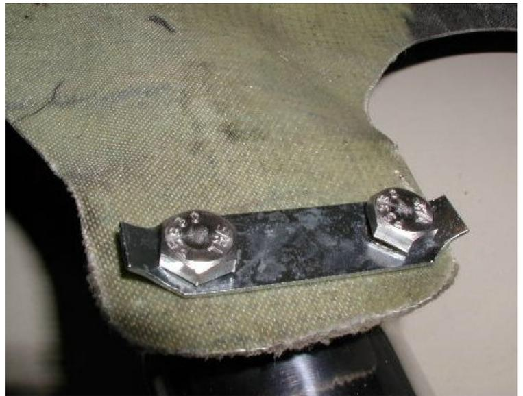
This picture shows the stock fender actually mounted on a bike with the tabs bent over to secure the bolts from coming loose.
