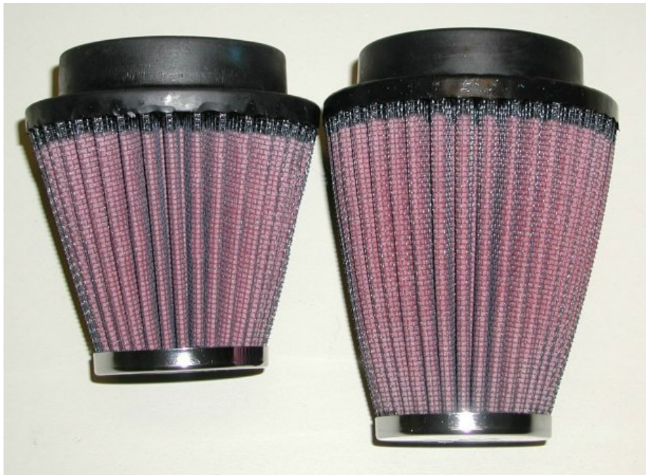
The modified filter is pictured on the left with the stock RC-1250 K&N on the right.
