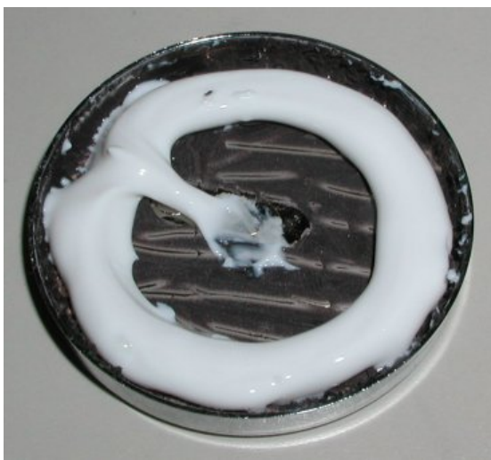
The silicone applied to the end cap.
