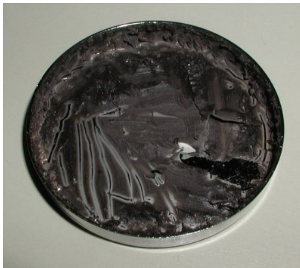
The end cap after all the old filter is removed.
