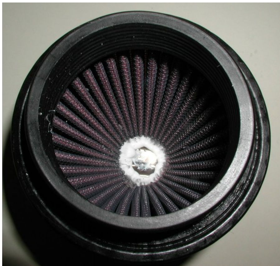
The bead of silicone inside the filter.
