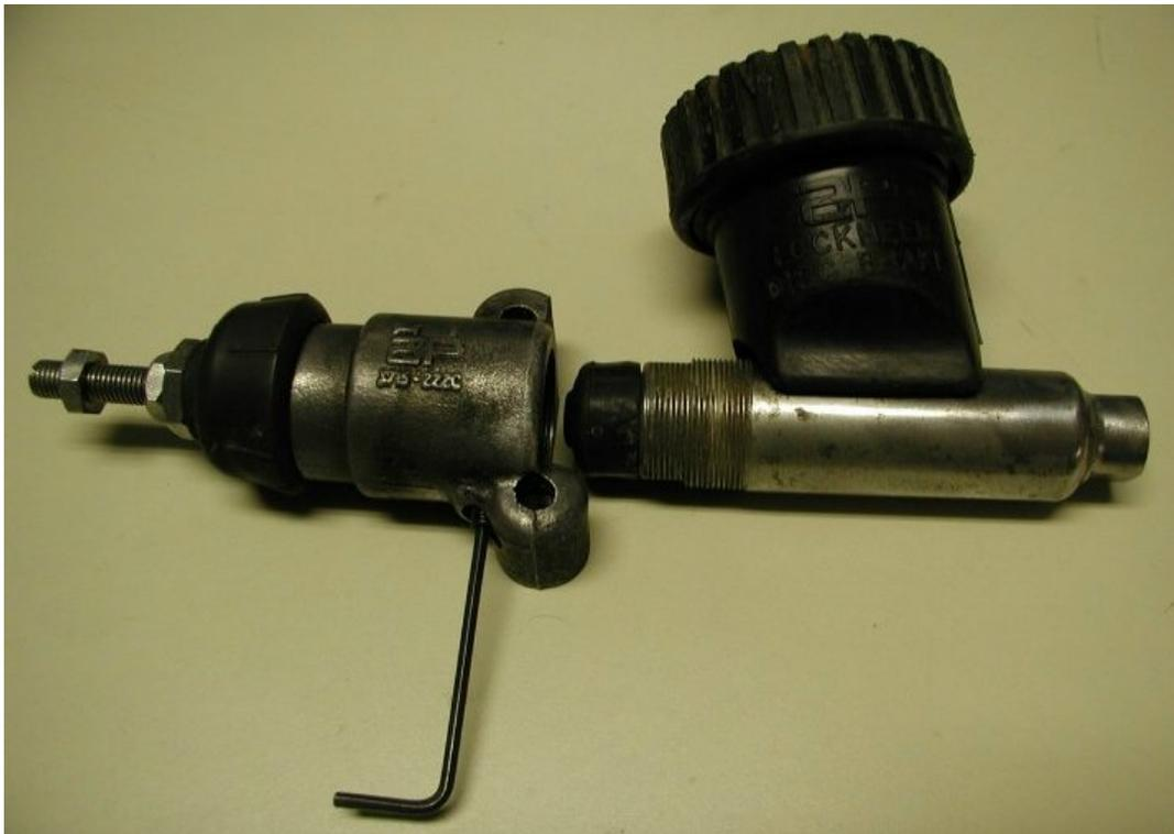
**Second**, thoroughly clean all parts making sure the cylinder bore is smooth and clean, the piston's three holes are open and clean, etc.
