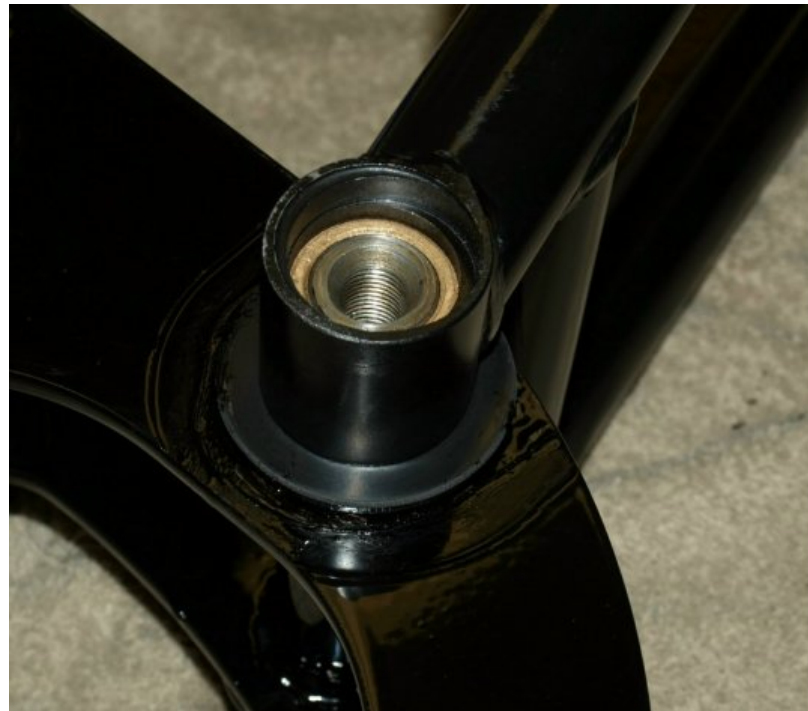
The bushings installed in the swingarm with the swingarm mounted to the engine cradle.
