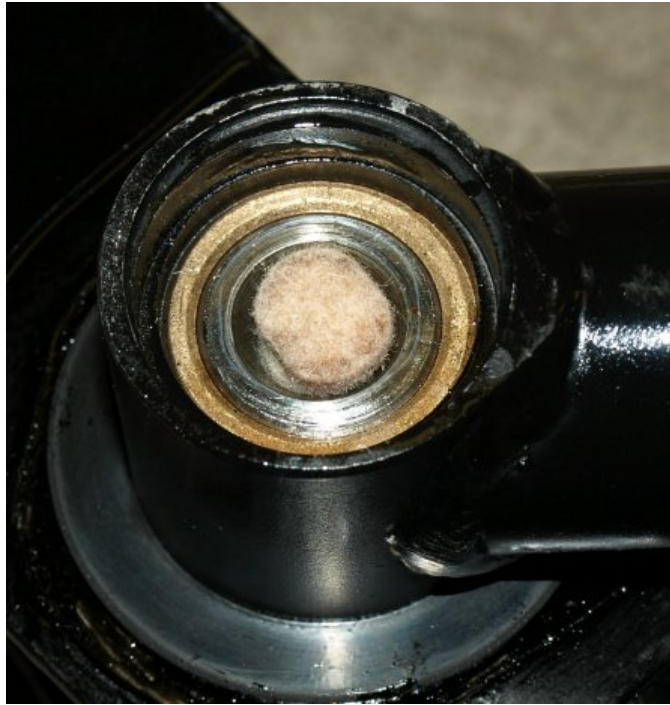
The oil wick (12) inserted into the swingarm spindle.
