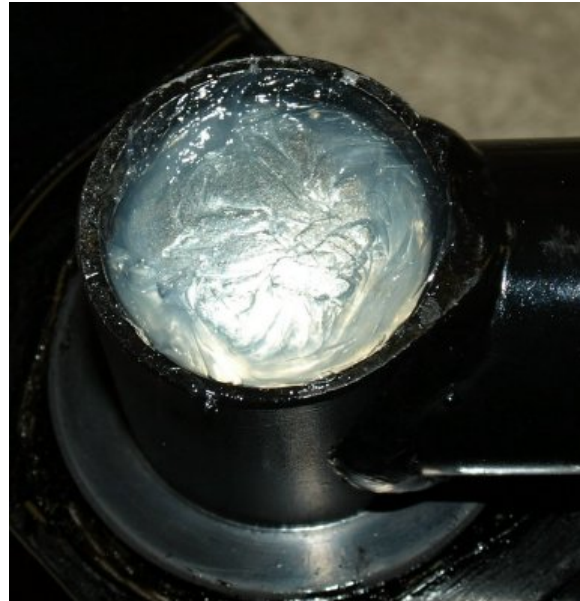
The welch plug sealed with silicone adhesive.
