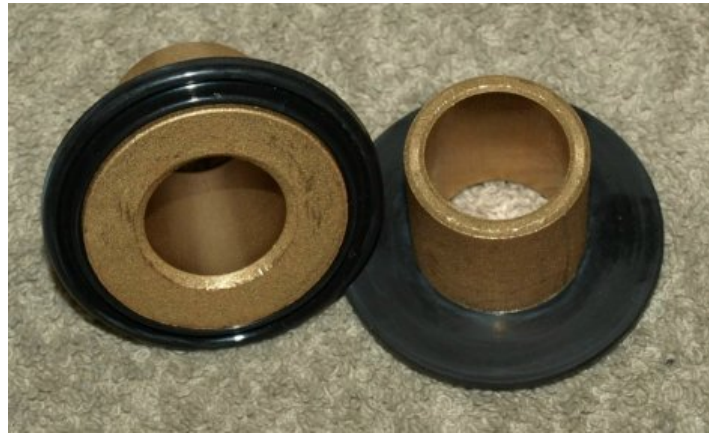
The MK3 swingarm bushings with the oil seals installed.
