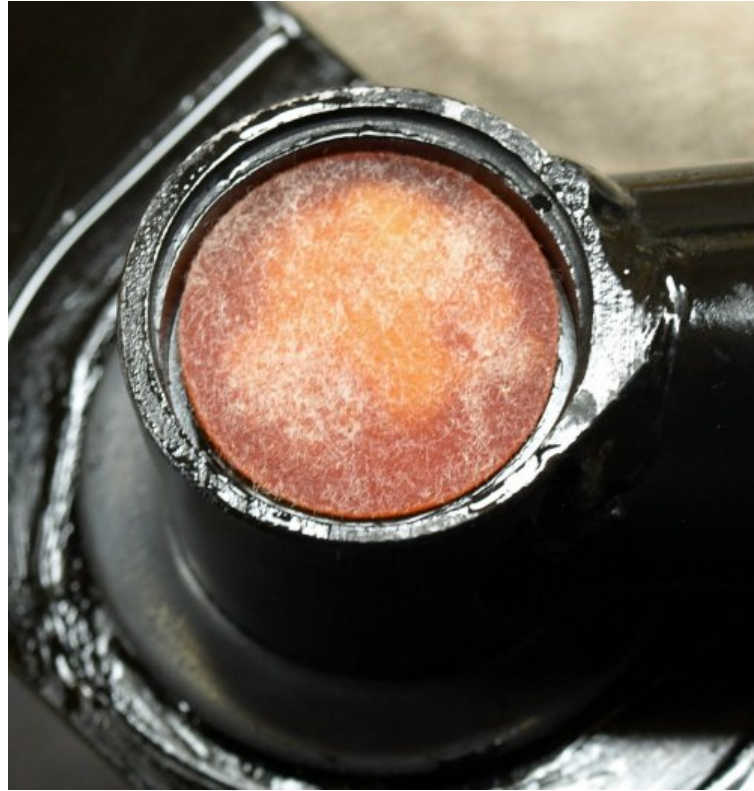
The oil disc wick (3) in the spindle.
