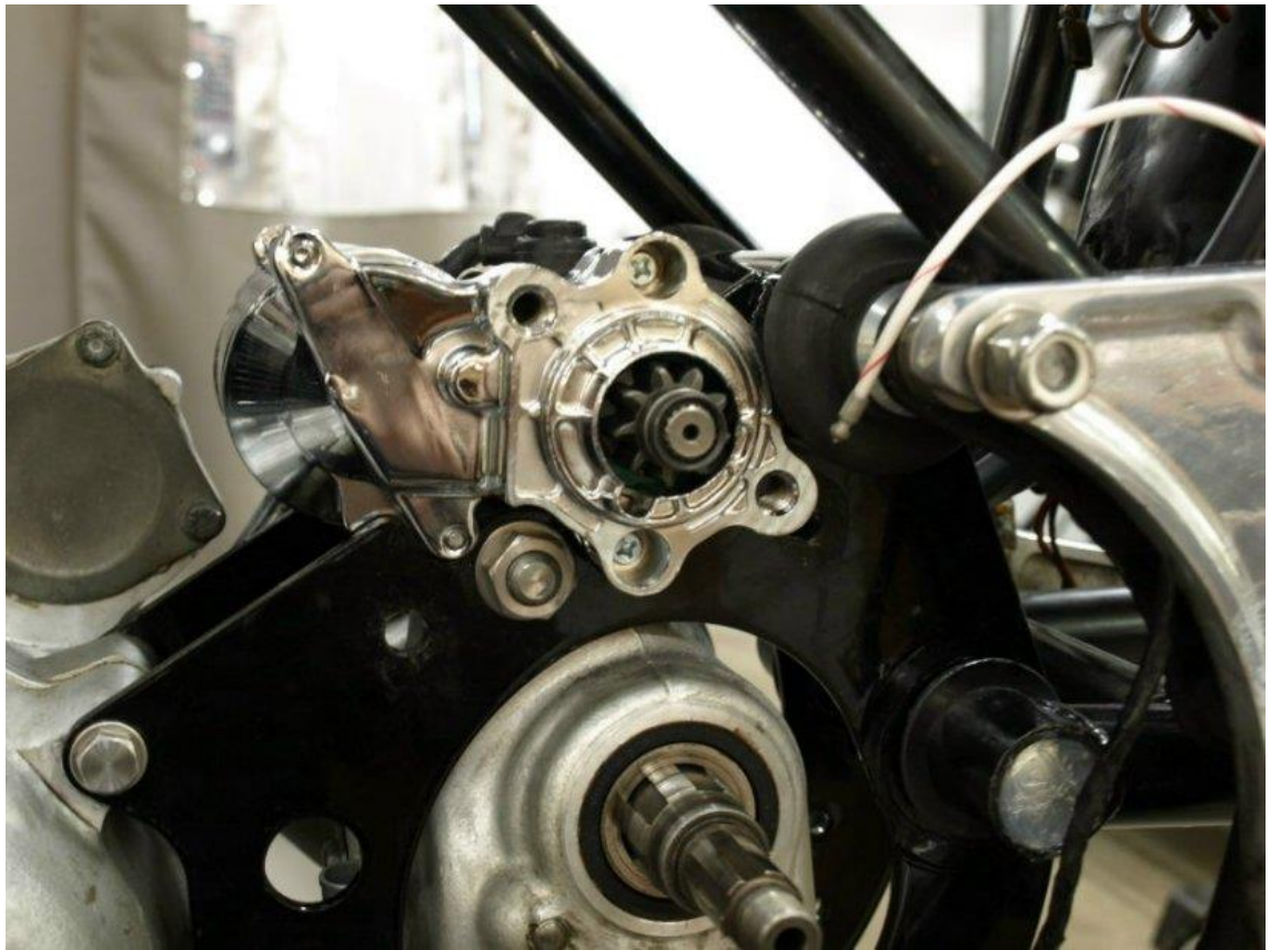
The left side of a properly installed starter.
