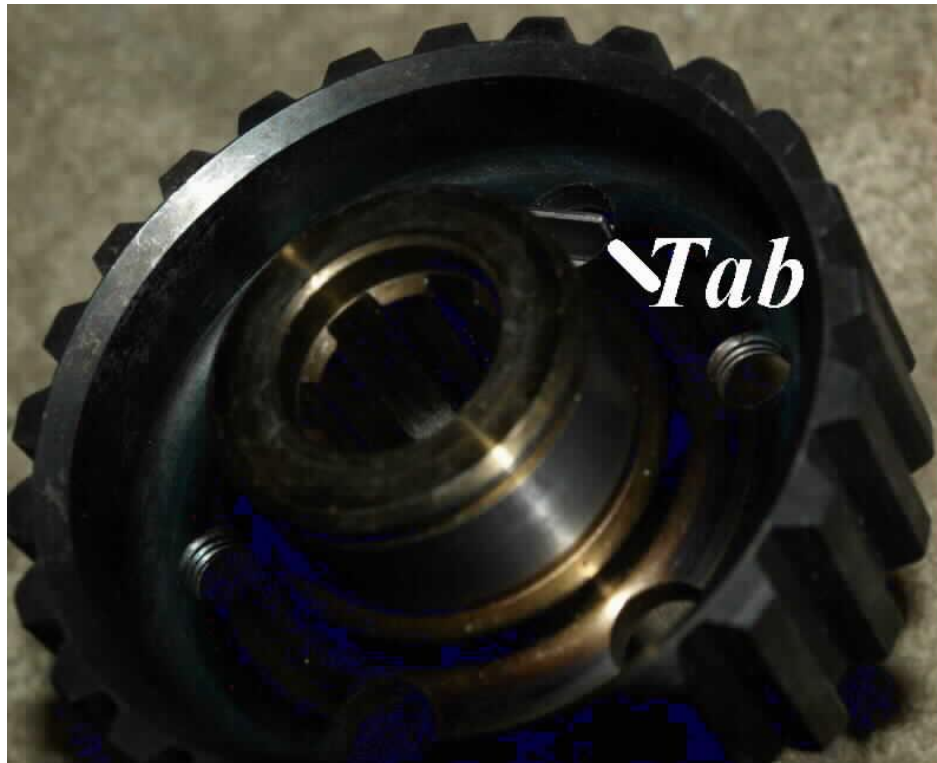
The tab sticking through the clutch center.
