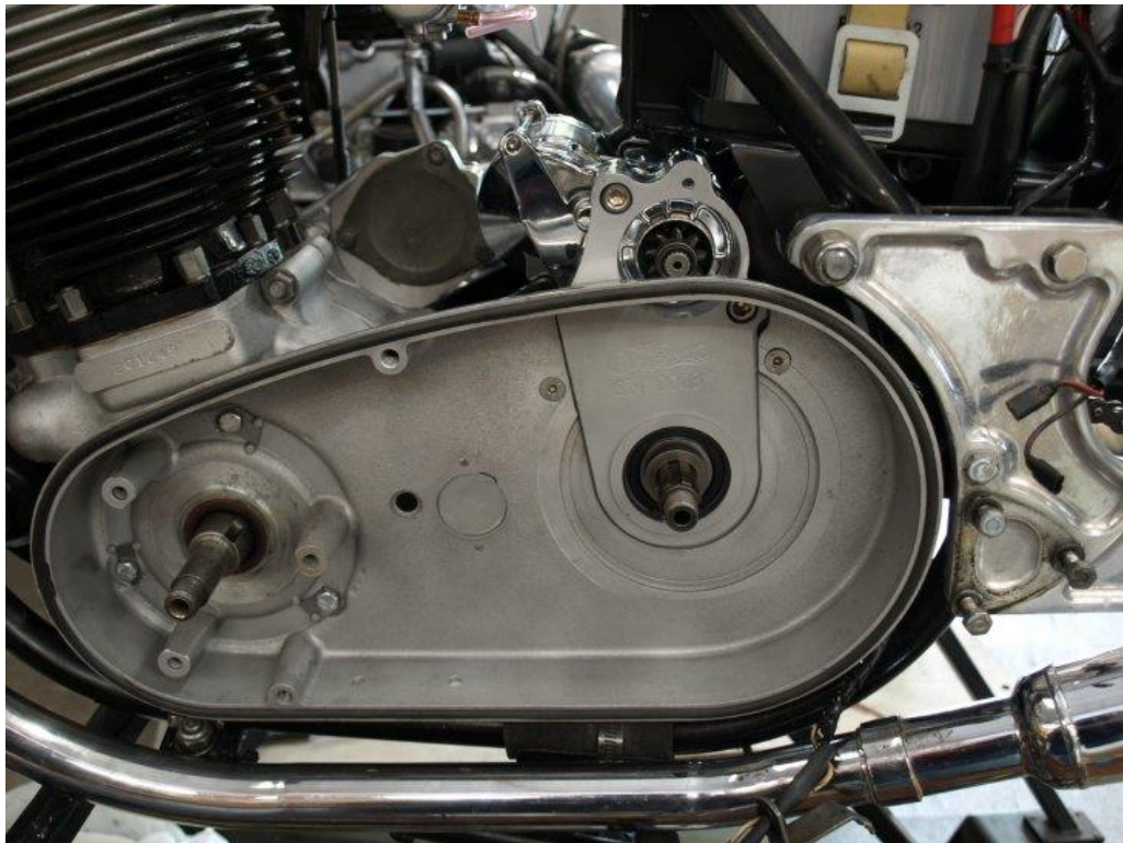
The inner primary case installed.
