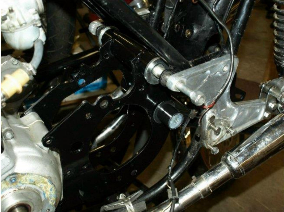
Engine cradle temporarily in place.
