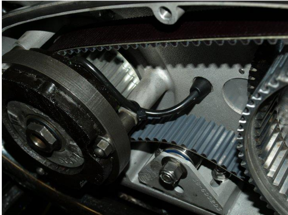
Alternator installed, note the wire tie location.
