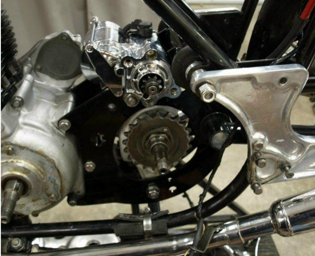
A 21 tooth sprocket installed on the gearbox.
