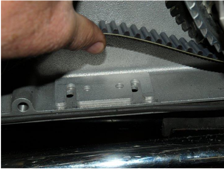
One shim in it's proper position.
