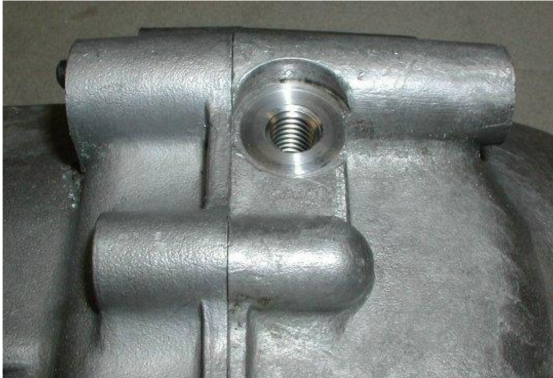
The finished refurbished drain hole.
