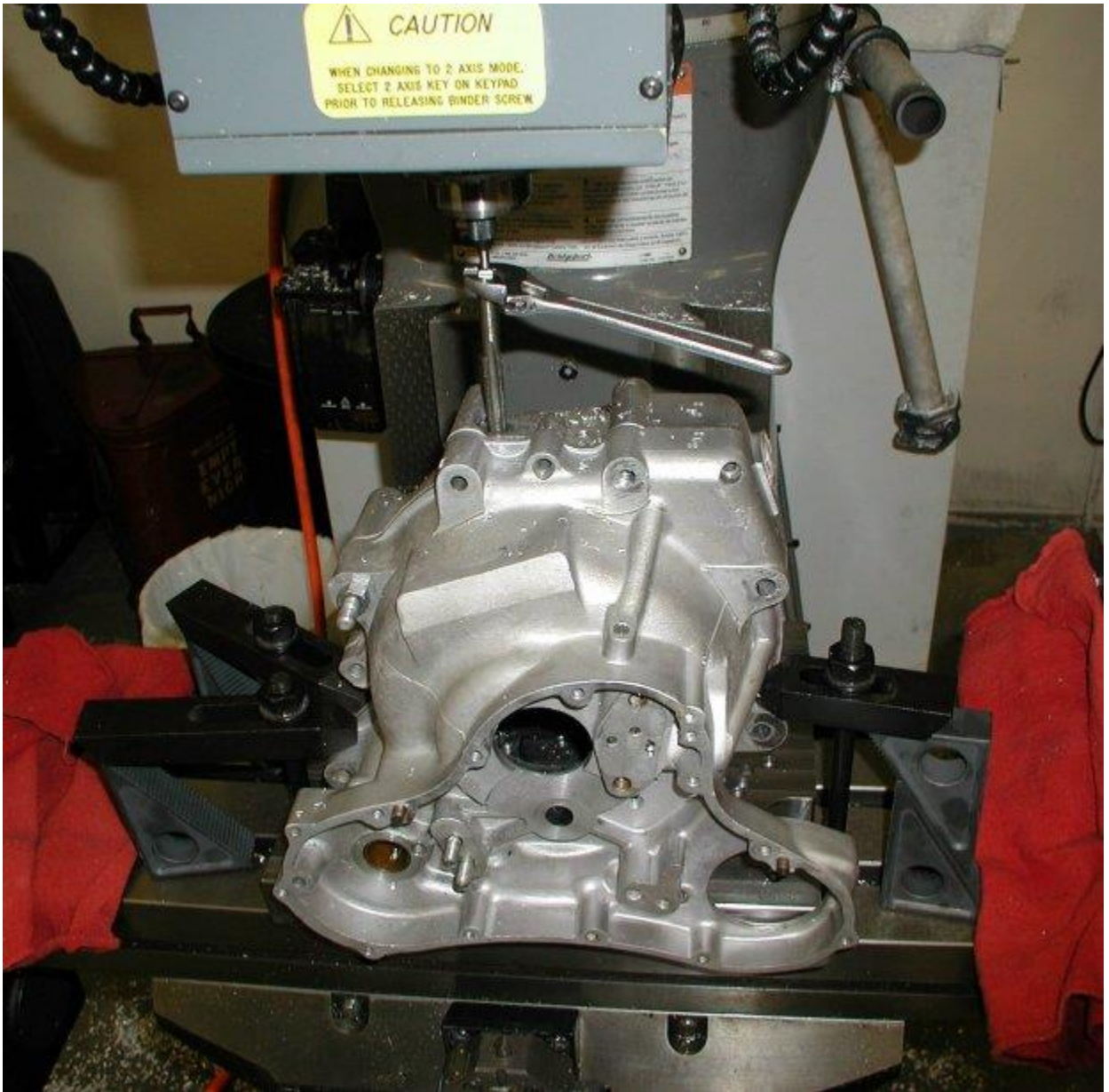
Tapping the drain hole.
