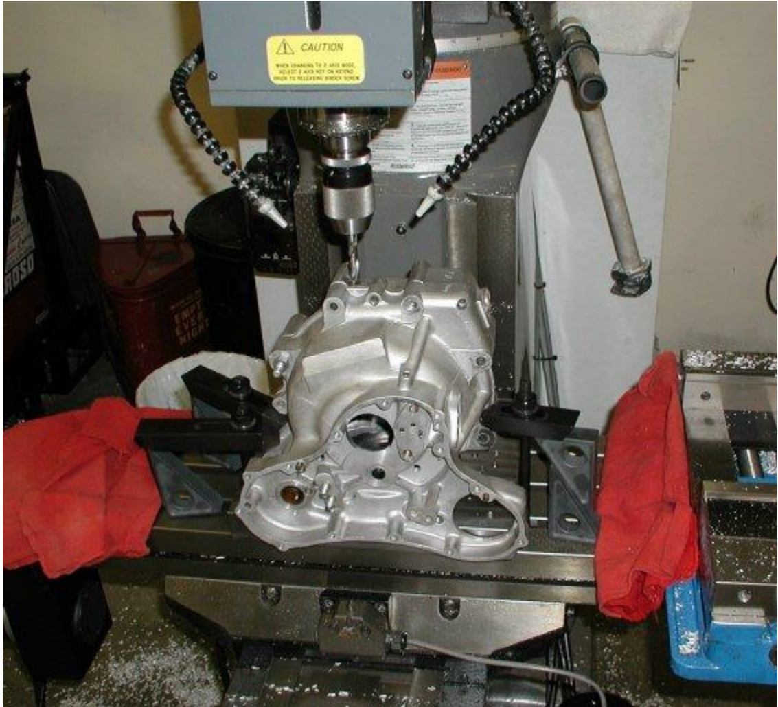
The secured cases with the 25/64 drill.
