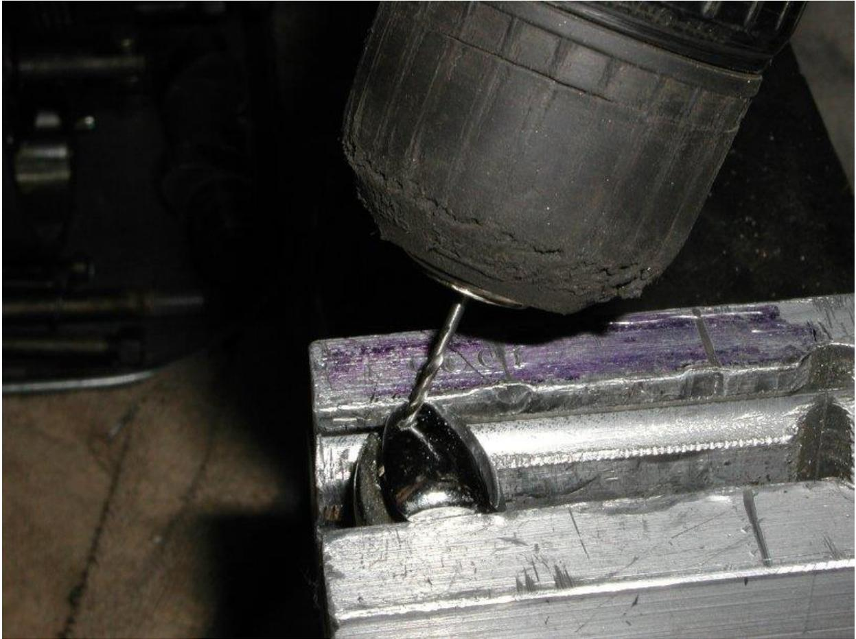
Drill through both sides of the weight using 1/16" drill.
