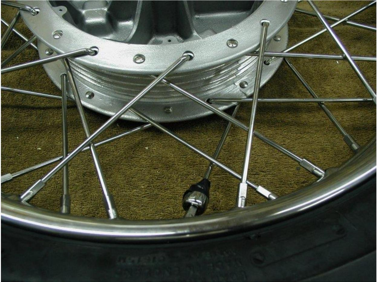
When you get the wheel back from having the tire mounted the weight should be taped to the spoke.
