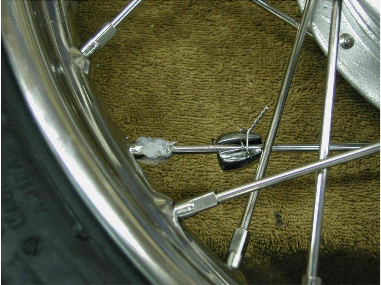
Safety wire the weight and put silicone sealer around the nipple.
