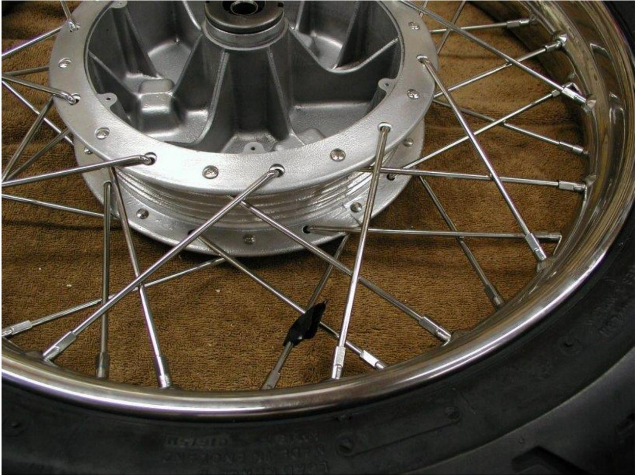
Remove one weight at a time, if more than one weight is used, and leave the tape on the spoke, so you know from which spoke the weight came off.
