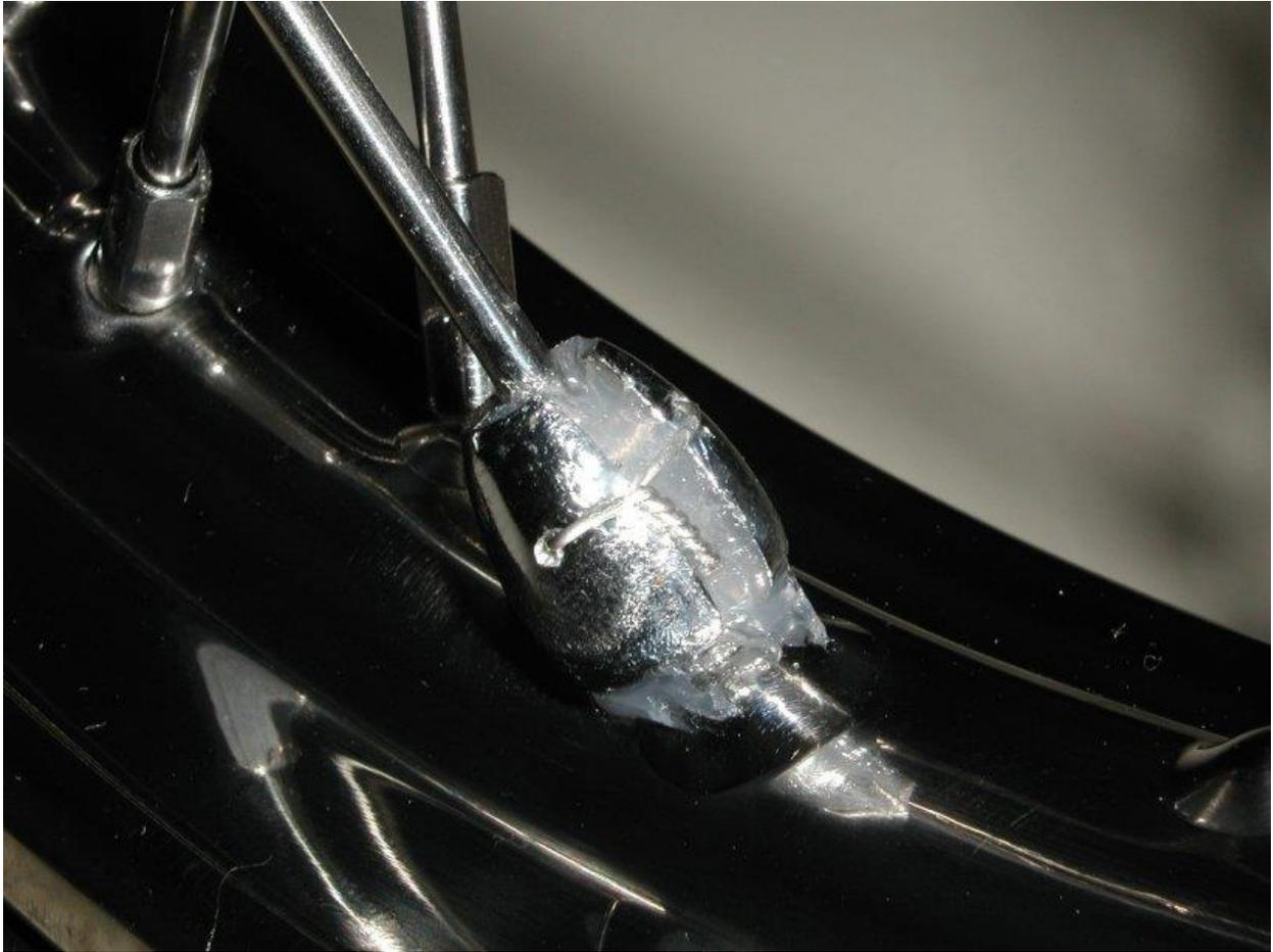
Slide the weight down on the nipple and bend the end of the safety wire into the silicone. You can clean up the excess silicone after it hardens.
