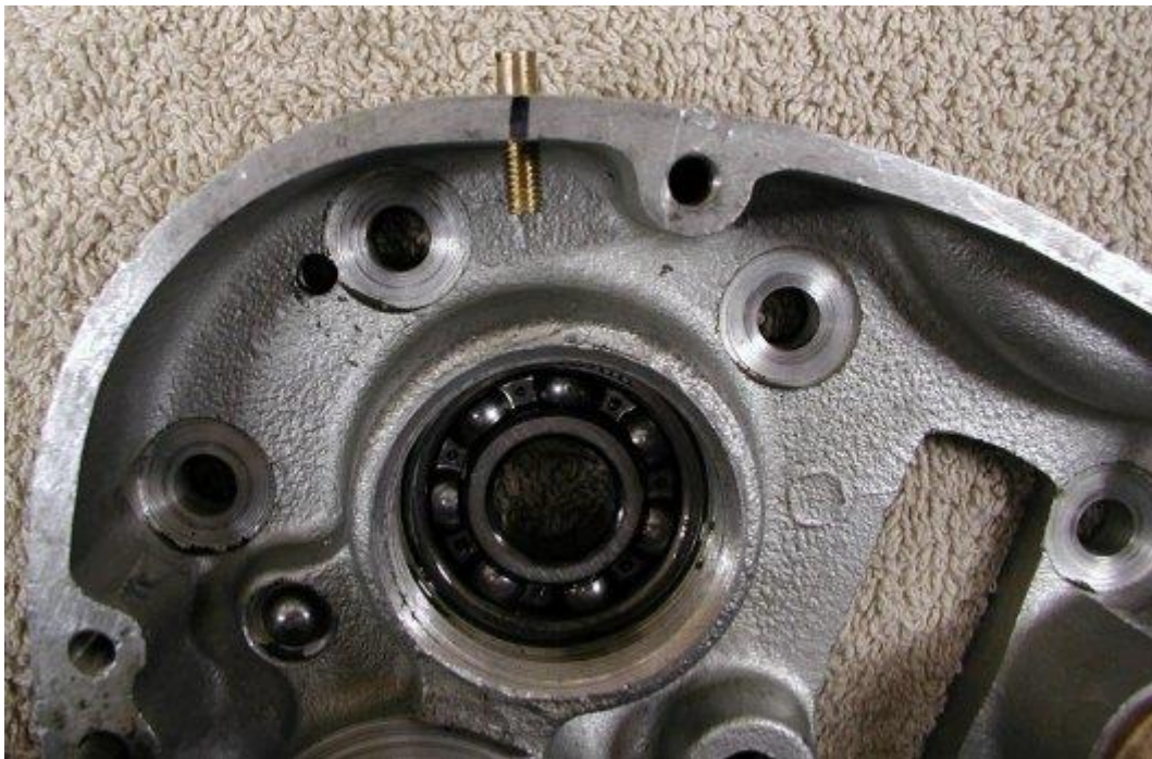
A picture of the breather installed on the inner gearbox case.
