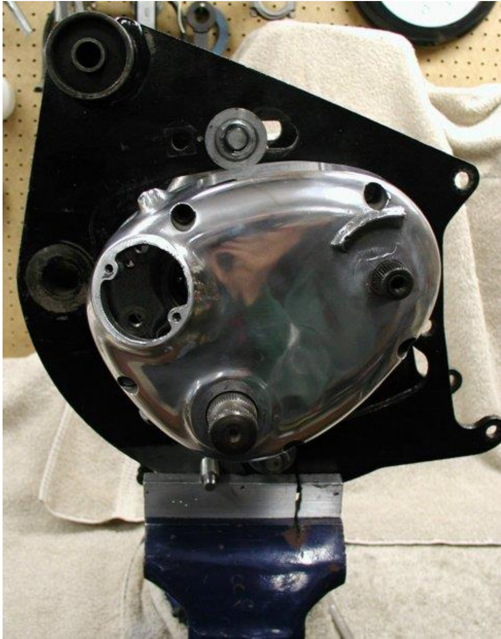
Gearbox mounted to the rear engine cradle and bolted securely in a vise.
