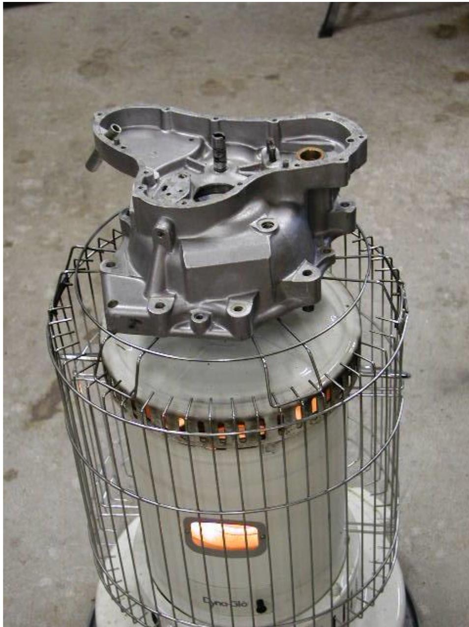
If you have a kerosene space heater as pictured, this makes a simple way of removing the crank bearings. If not you may want to think about acquiring one since they are handy, not that expensive and readily available at most large hardware stores. I have been using this type of heater for years to bring my shop up to a pleasant working temperature in the winter. My shop is heated with electric heaters which I keep at around 50❖F to
