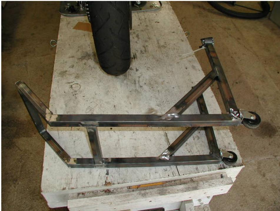
For the top of the stand that contacts the swinging arm, I actually took a section of 1 5/8" exhaust pipe that I had laying around, cut it lengthwise and welded it to the top. You could take any pipe of the desired diameter, cut it lengthwise and weld it to the top. If the pipe you use is thick and does not bend easily, make sure it is a larger diameter than the swinging arm. I then drilled a hole just under the welded pipe halves to be able to wire tie the rubber buffers to the top.
