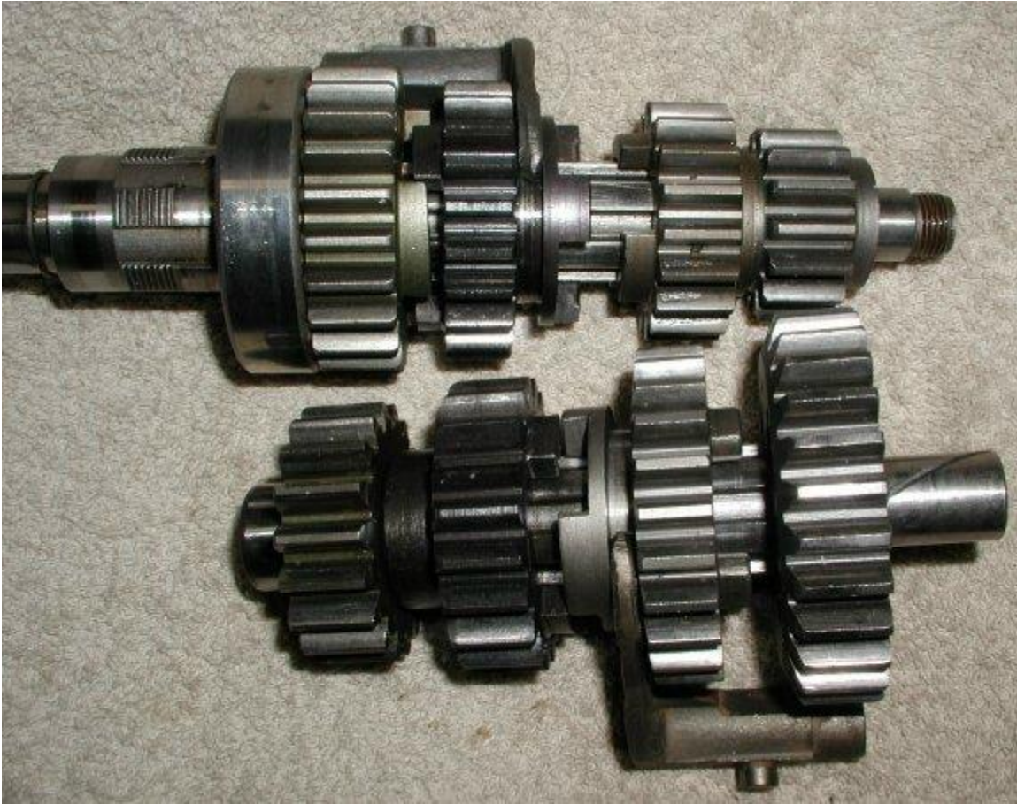
The gears on their shafts.
