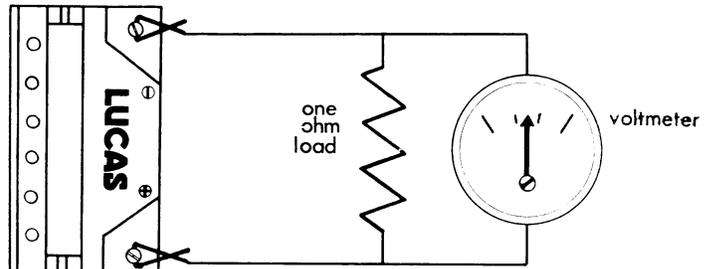
Fig. 65 High rate discharge test
