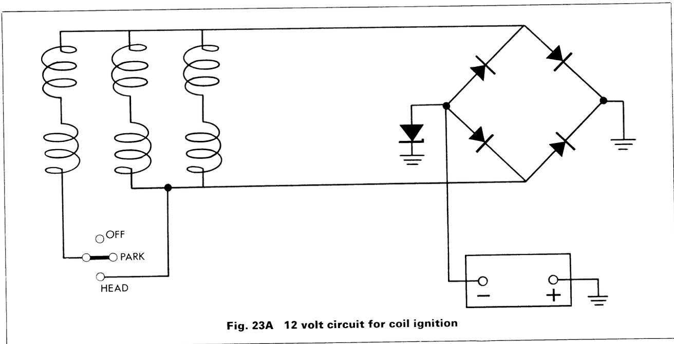
**Fig. 23A 12 volt circuit for coil ignition**
