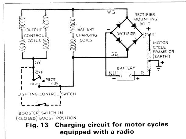
**Fig. 13** Charging circuit for motor cycles equipped with a radio
