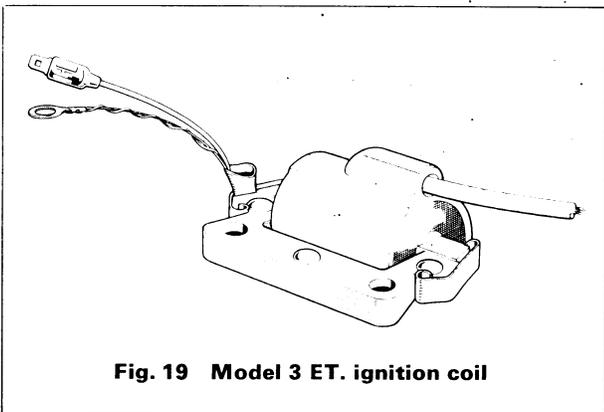
Fig. 19 Model 3 ET. ignition coil
