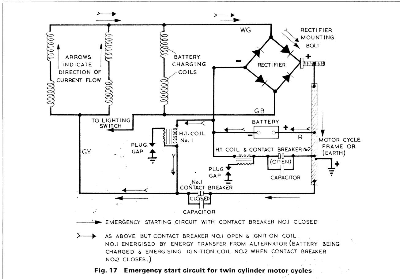
Another feature of the system is that the coil No. 2 eventually comes into operation during emergency starting, so that after a few seconds running on one cylinder, number two cylinder cuts-in and the engine functions as a normal twin-cylinder unit. It will not operate on both cylinders after a few more seconds because the rising battery voltage causes misfiring on the one cylinder.
