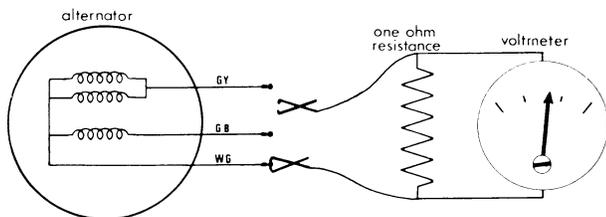
Fig. 67 Alternator output test
