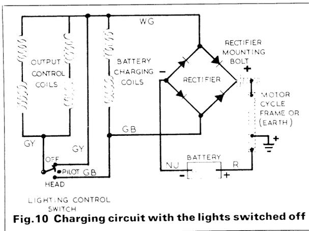
**Fig. 10** Charging circuit with the lights switched off
