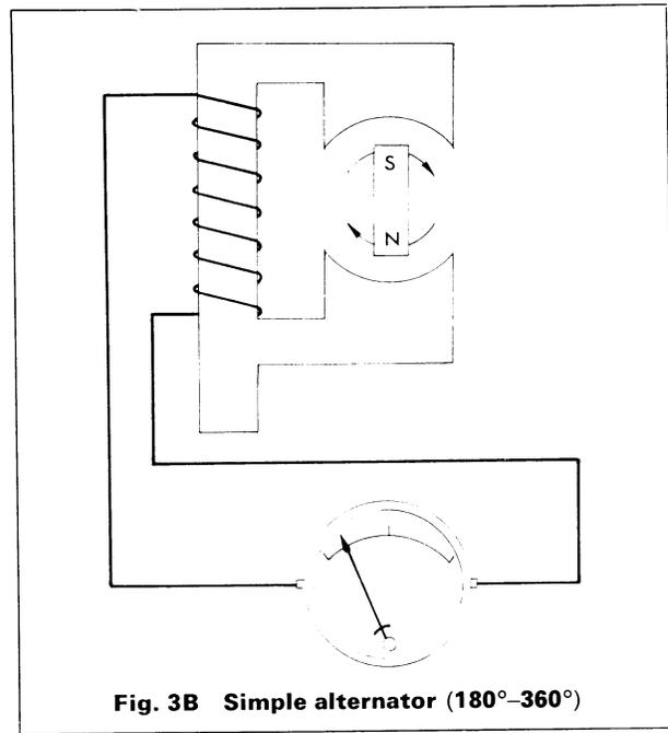
Fig. 3B Simple alternator (180°-360°)
