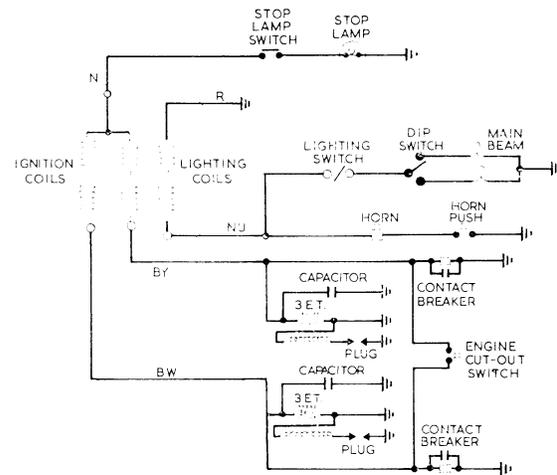
Fig. 21 A.C. ignition circuit for twin contact motor cycles
