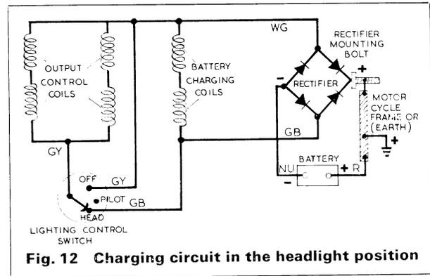
**Fig. 12** Charging circuit in the headlight position
