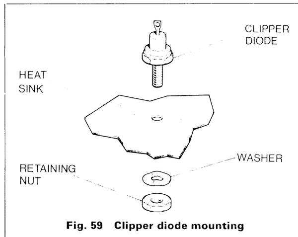
Fig. 59 Clipper diode mounting
