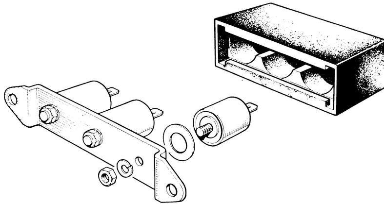
**Fig. 31 Capacitor pack model 2CP**
