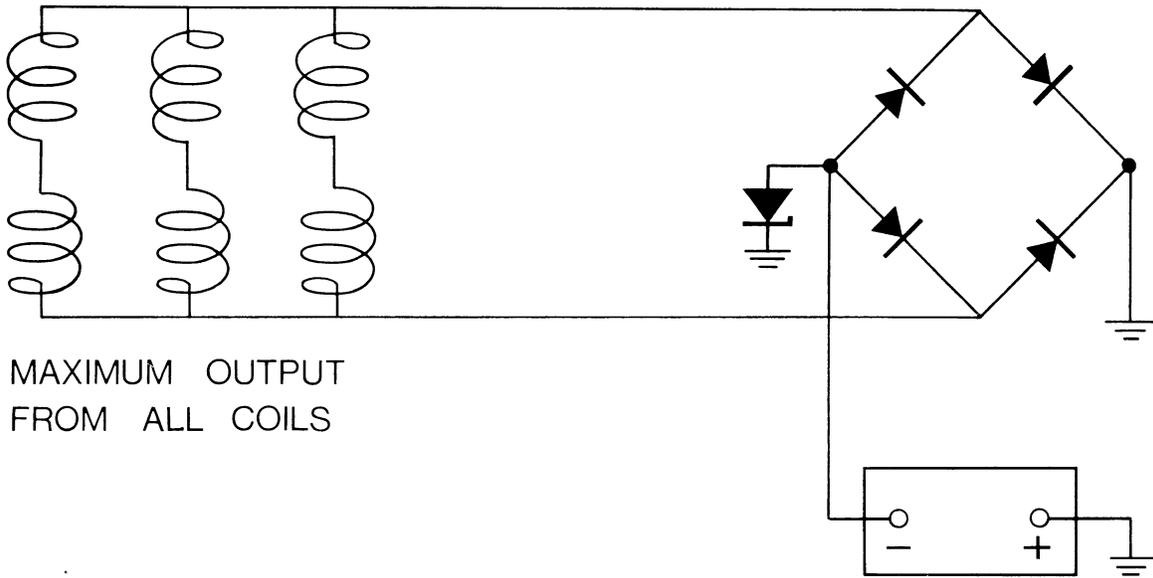
**Fig. 24 12 volt circuit connected for continuous maximum output**
