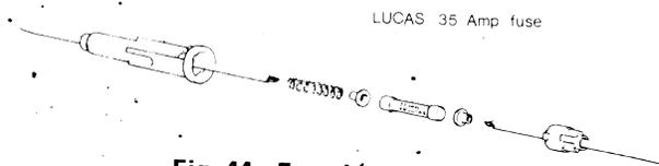
**Fig. 44 Fused battery lead**
