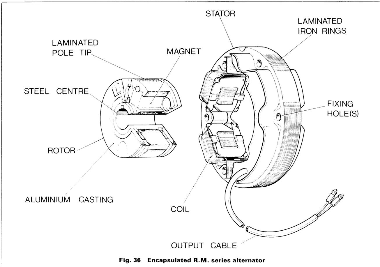
Fig. 36 Encapsulated R.M. series alternator
