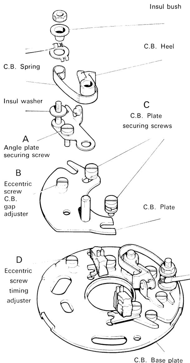
Fig. 28 Contact breaker model 6CA
