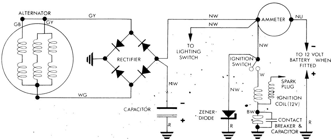
**Fig. 25 Basic capacitor ignition circuit**
