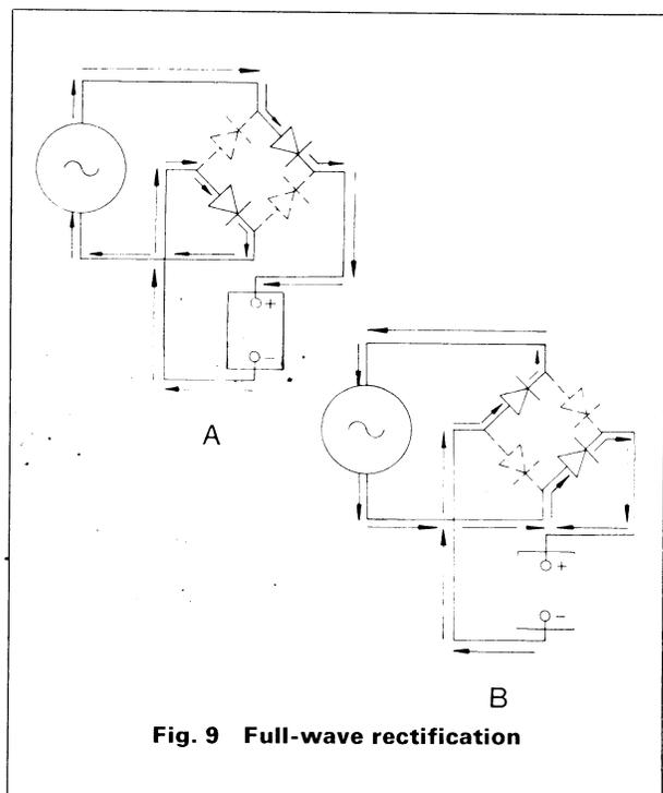
current is flowing in a clockwise direction; the right-hand illustration (B) an anti-clockwise direction. With this arrangement the full output from the generator is utilised. That is, both the positive half waves and the negative half waves are used to charge the battery, shown by the graph C in Fig. 6, by inversion of the negative half wave.
