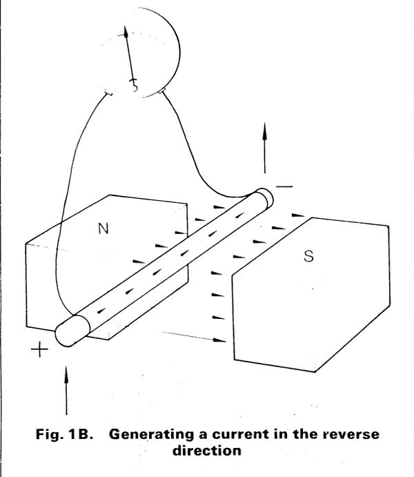
Fig. 1B. Generating a current in the reverse direction
