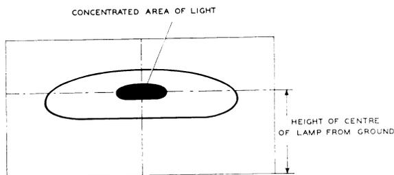
**Fig. 41 Headlight adjustment**
