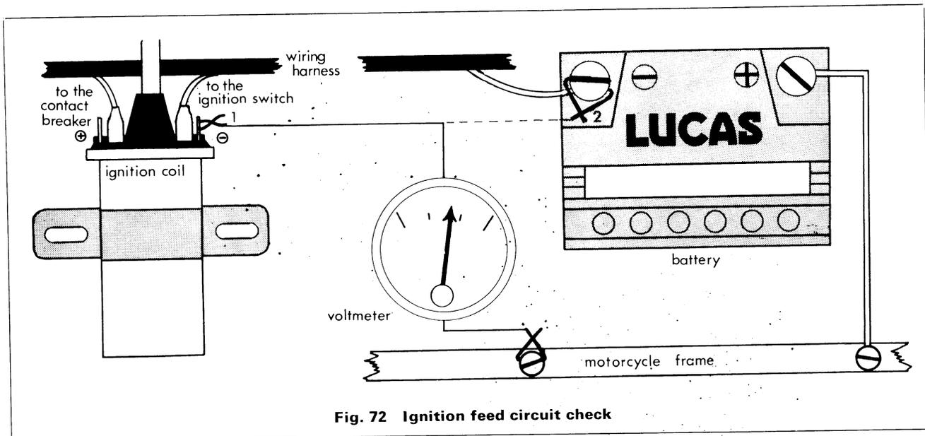
**Fig. 72 Ignition feed circuit check**
