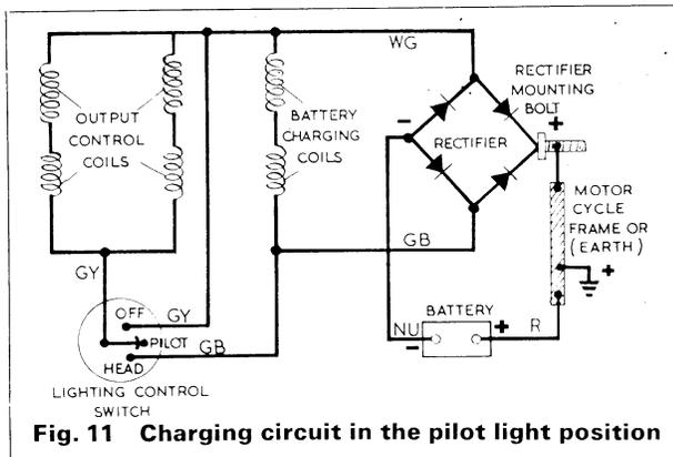
**Fig. 11** Charging circuit in the pilot light position
