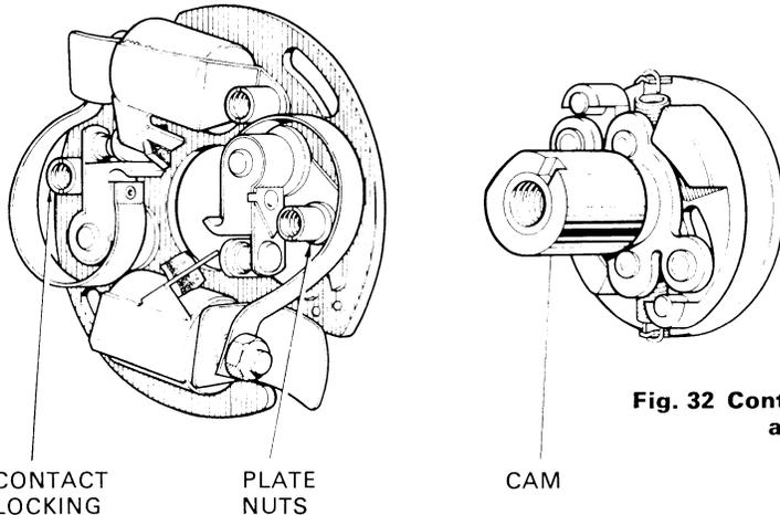
**Fig. 32 Contact breaker model 4CA and auto advance unit**
