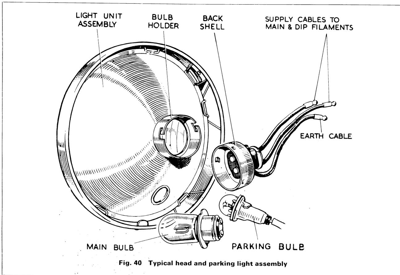
Fig. 40 Typical head and parking light assembly
