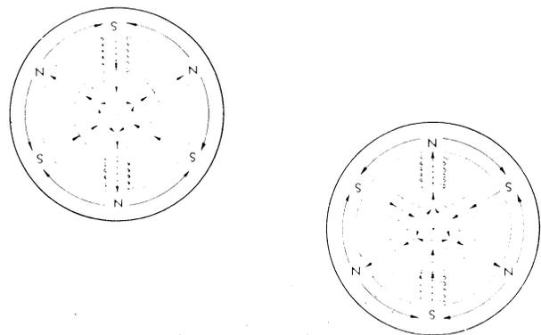
Fig. 5 Lucas alternator arrangement
