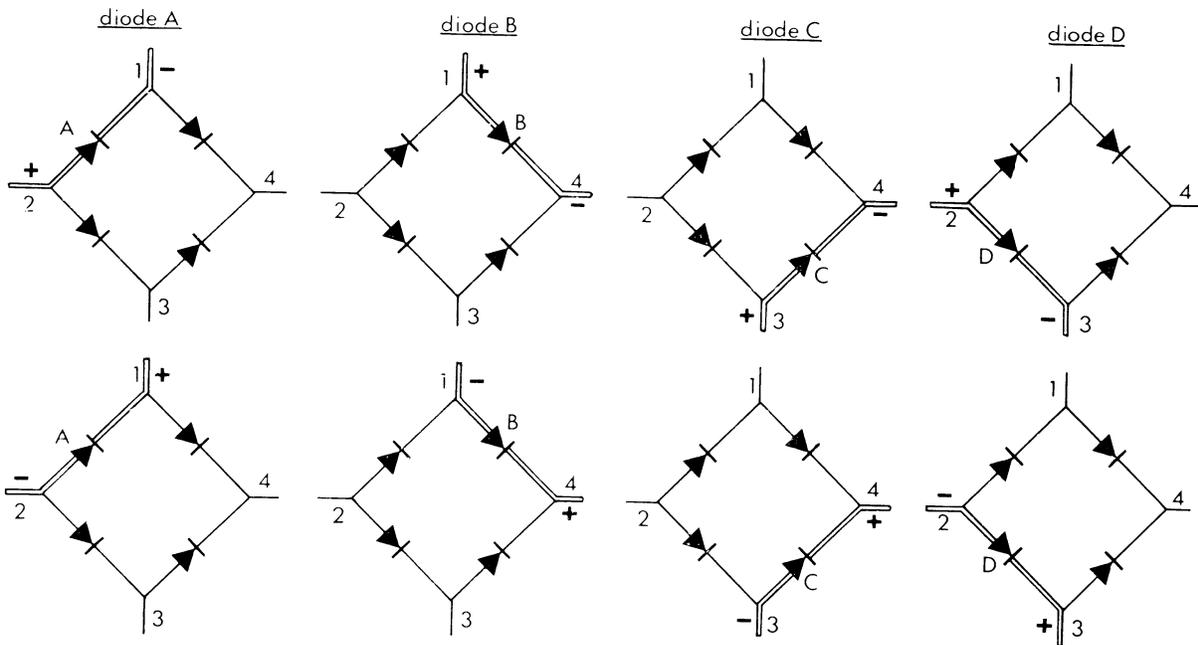
Fig. 69B Rectifier bench test (individual diode circuits)
