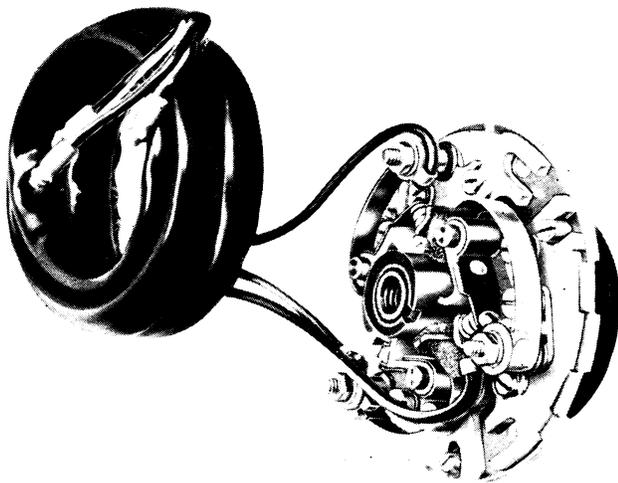
Fig. 29 Contact breaker model 7CA
