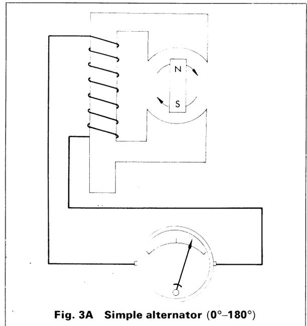
Fig. 3A Simple alternator (0°-180°)
