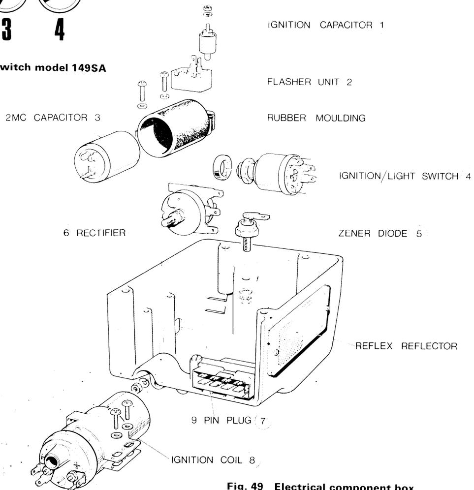
Fig. 49 Electrical component box
