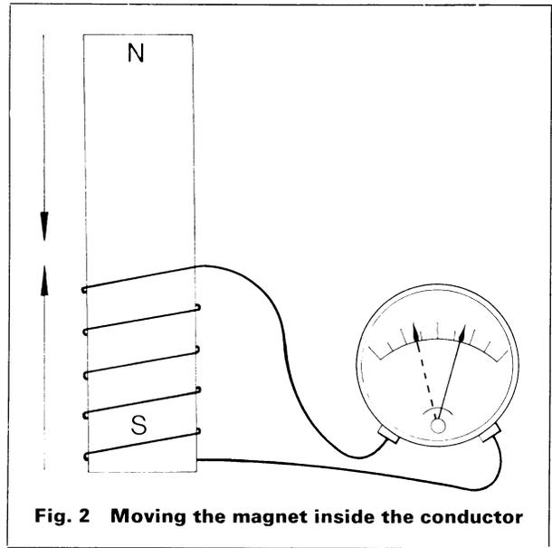
Fig. 2 Moving the magnet inside the conductor
