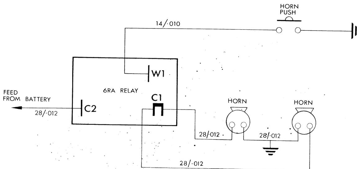
Fig. 61 Twin horn circuit
