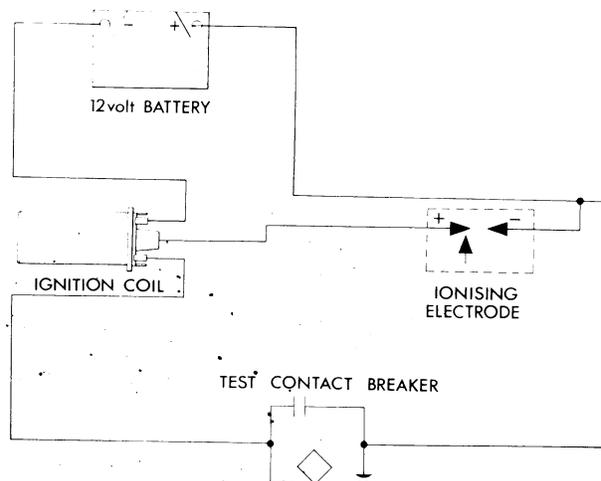
Fig. 75 Ignition coil bench test circuit
