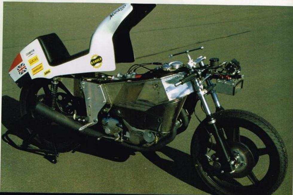
24 litre fuel supply then permitted under FIM F750 rules, as well as the six-pint oil tank for the dry-sump engine, located in the rear section of the frame. In this way, Williams was able to incorporate the same fuel load as in the '72 bikes, but reduce the centre of gravity and frontal aspect still further, in a bike 20 lb lighter than the old one, at 350 lb/159 kg dry.
