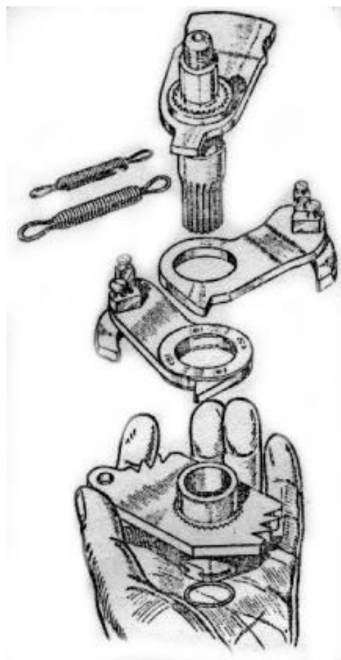
Fig. 38. Gear change mechanism
