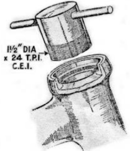
Fig. 42. Steering head ballrace extractor.
