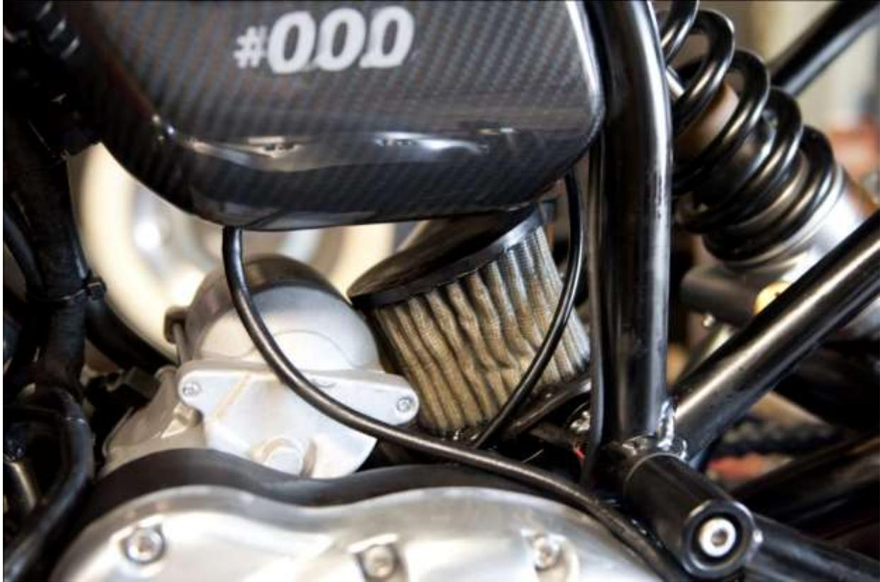
It is possible to remove the Air Filter without removing the AirBox.
