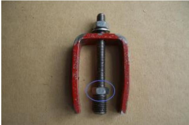
The lower nut is important to prevent the bolt from turning while compressing.
