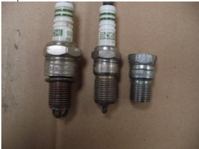
Knock out the ceramic and centre electrode (wear eye protection!) and drill out. I found it really hard to remove the ceramic centre and so used a TDC finding tool, enlarging the central hole to accept the bolt.
