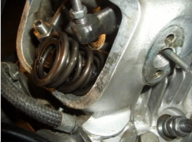
Once the spring is out, keep the rocker up with for example, a rubber band. You now have free access to the seal!
