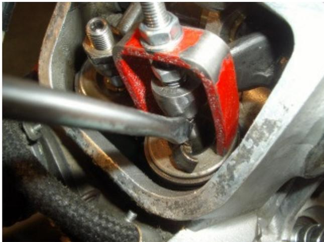
Remove Tool 1 (the threaded rod can be left in place). Next, if you don't mind fiddling with spring washers and shims in tight places; just remove the rocker arm completely. But if you prefer to keep the rocker arm in the head, go to the next step: Loosen Tool 2 and turn it 180 ° so that you can lower the valve against the piston (it was a few mm past TDC, remember?):
