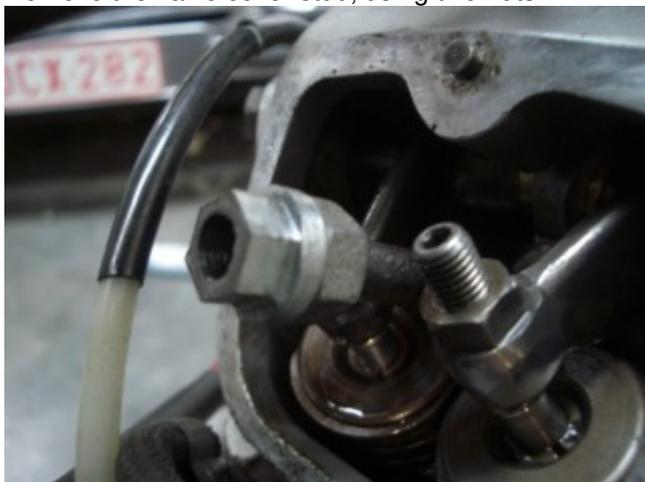
Now remove the valve adjuster and install Tool 1. If you have mushroom adjusters, use a thin rod in place of the rocker shaft so that you can lift the rocker up sufficiently to remove the adjuster bolt.
