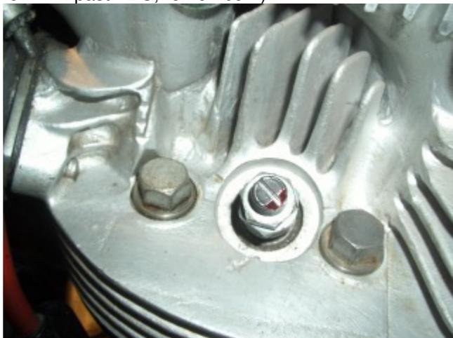
Replace the temporary 12mm rocker shaft with a 4mm thin rod. This will allow you to push
