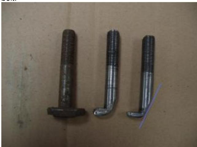
The chamfer is very important, as it enables the piece to easily slip through the plug hole:
